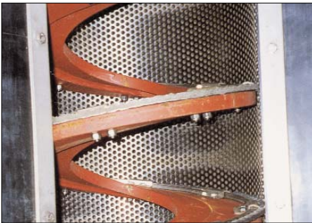
Durable spiral brush keeps the screen clean.
