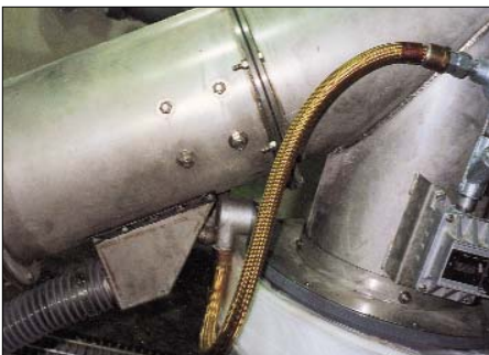
Close-up view of the new drain box with optional explosion-proof wiring.
