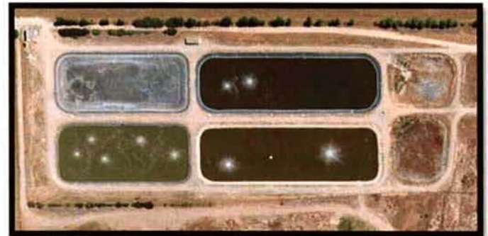
NCSD's Southland WWTF discharges roughly 580 AF/yr to percolation ponds. It is unclear whether this water recharges the groundwater basin.
