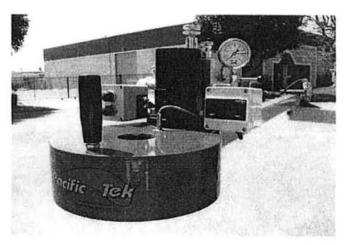
Turns valves with adjustable torque from 50 to 800 ft.lbs.
