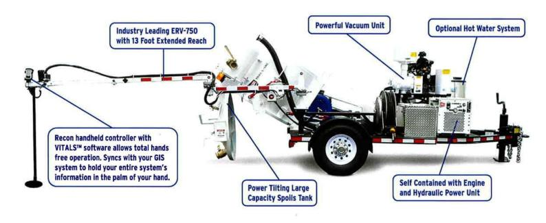
Patented automatic shutdown • Valve identification • Right hand/left hand I.D.
