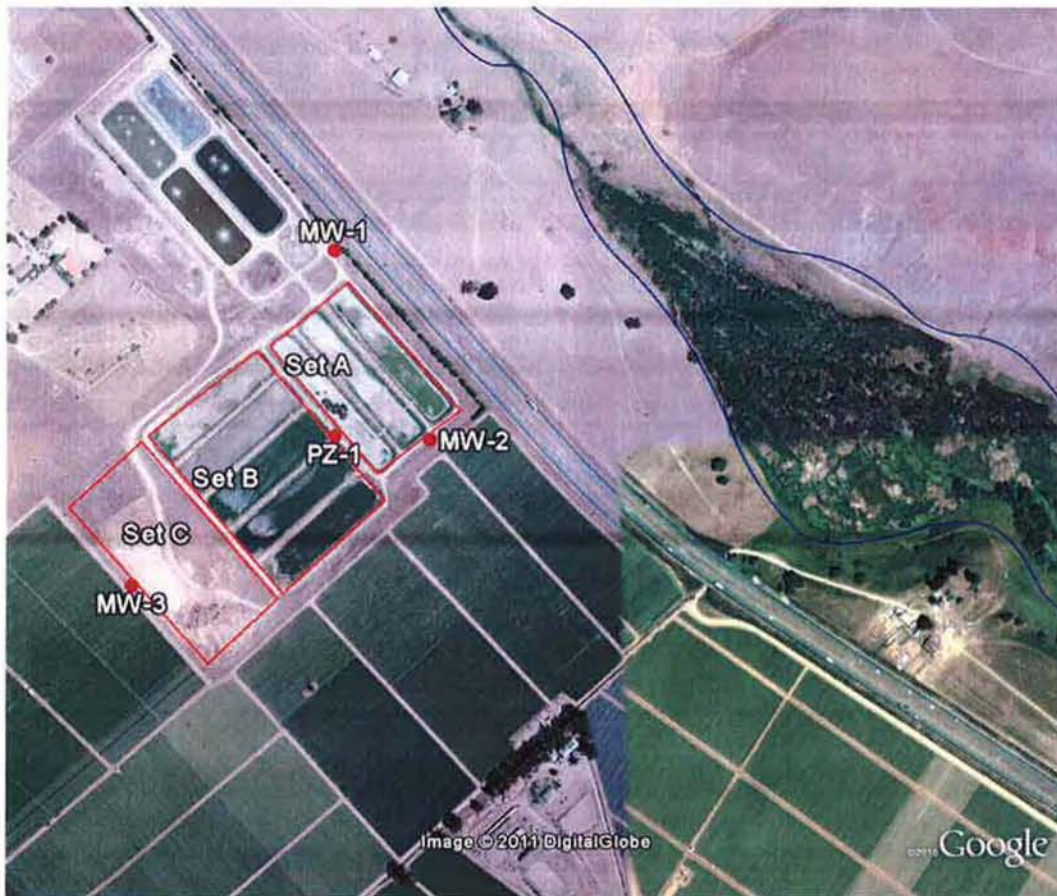
Figure 1. Map of Existing Two Sets of Percolation Ponds (Sets A and B) and Proposed Third Set of Ponds (Set C) at the Southland Wastewater Treatment Facility
