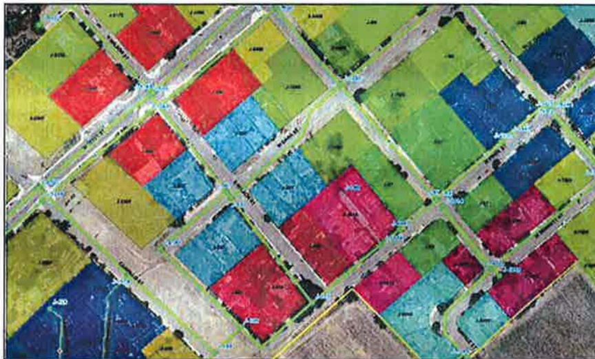
Figure 3. Screenshot of the water demand layer and exported WaterCAD model from the 2012 Model Update project recently completed by RICK and MKNA. A similar process will be followed for the Blacklake Sewer Master Plan.
