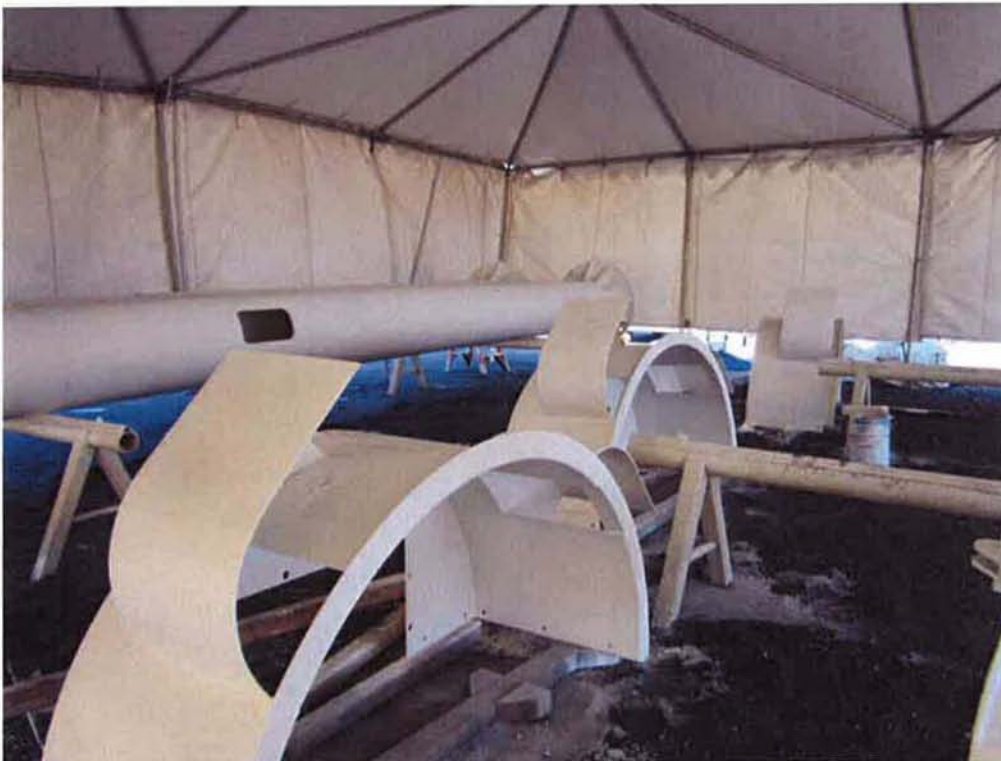
Clarifier mechanism parts after being primed.
