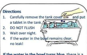
If the water in the bowl turns blue, there is a leak in the tank.
