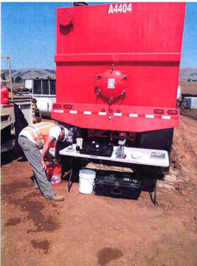
Wyo-Ben (mud engineer) on site testing mud samples using a filter press and viscometer.
