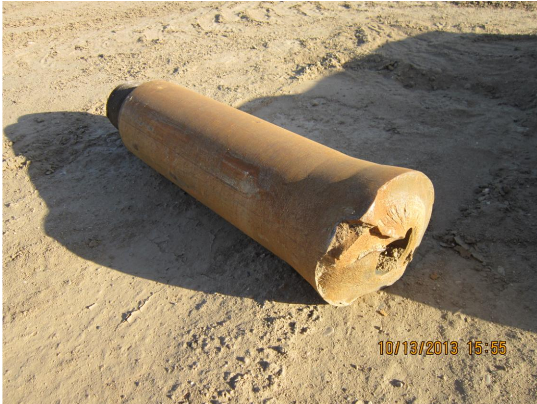
One of the failed adapters from the 42-inch drill.
