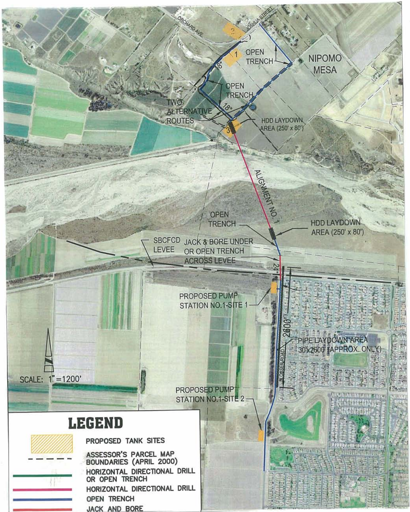
FIGURE 4 Pipeline Route and Project Facilities
