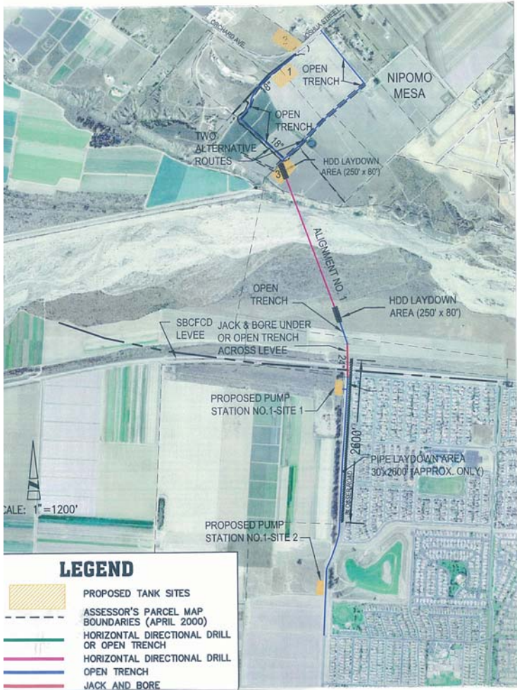
FIGURE 4 Pipeline Routes and Drain Facilities
