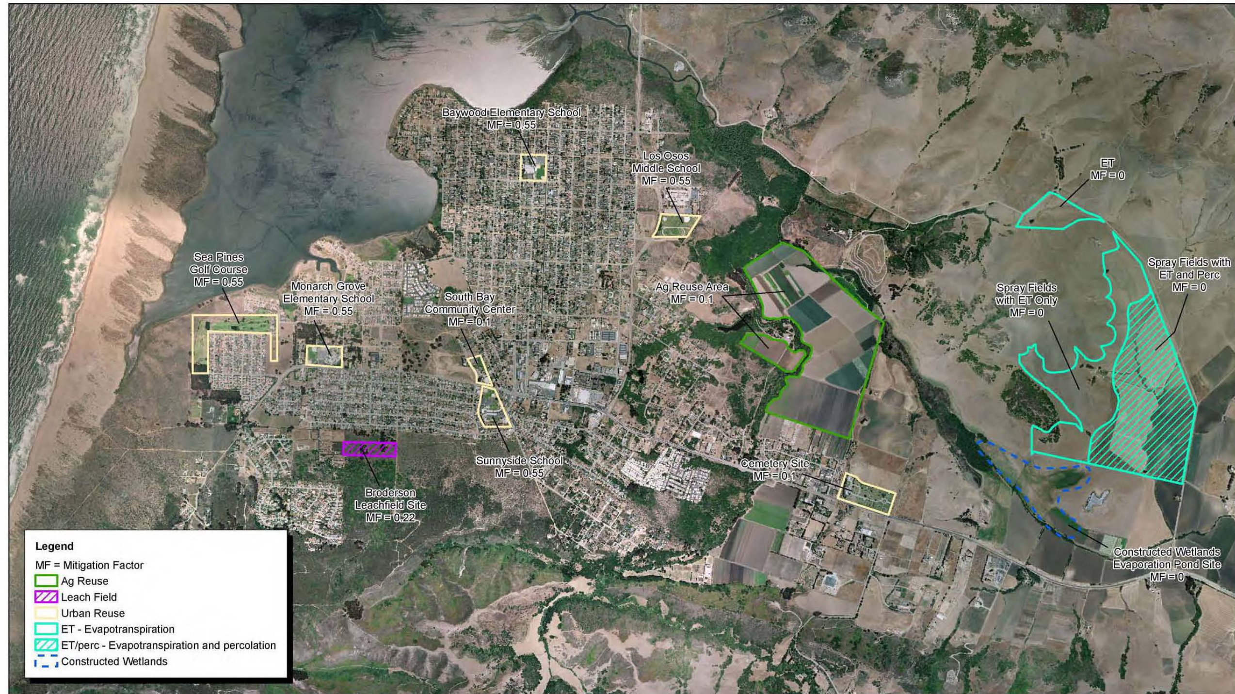
Figure 5.4 Effluent Disposal and Recycled Water Reuse Alternatives
