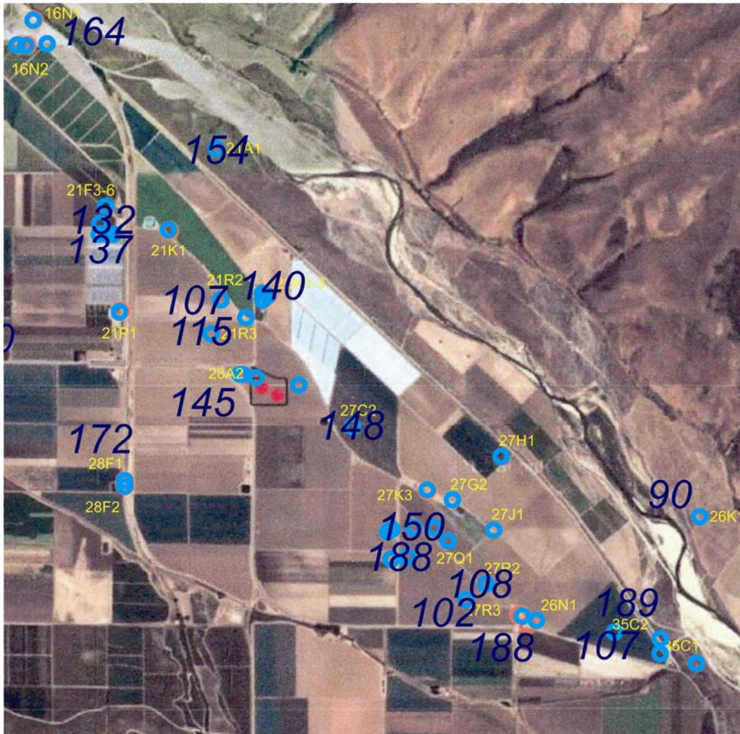
Figure 7. Sand thickness map, suffix of state well number (yellow text), wells (blue circles), and uppermost sand thickness (dark blue numbers, in feet from ground surface).
